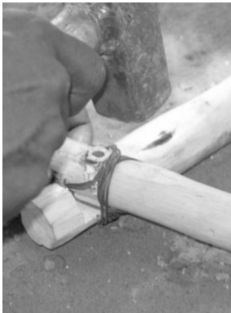
Figure 5.41 Circular hinge housing or sheath being inserted into the support frame of the tipper.
