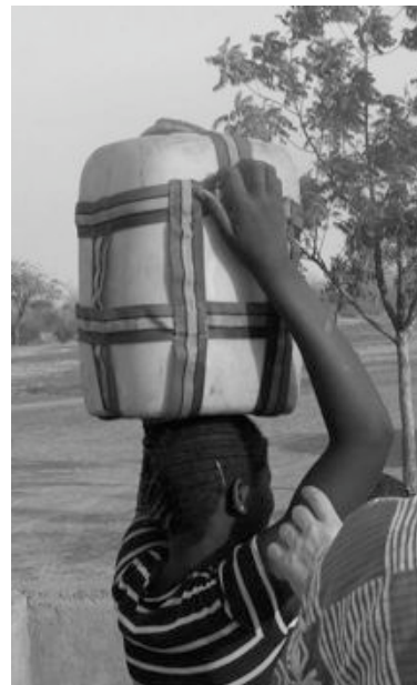
Figure 5.12 Testing of a jerry can holder (“porte-bidon”) made from nylon webbing sewn around the container to facilitate grasping and manipulation.
