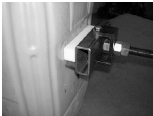
Figure 5.19 A close-up view of the external pressure plate on the handle (white piece) to be welded to the container.
