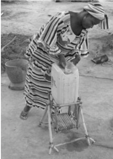
Figure 5.42 It is important before fabricating tippers to take measurements from containers when they are full (and thus expanded). This will assure easy placement and removal of the container in the completed tipper.
