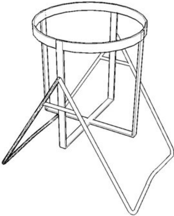
Figure 5.33 Basic design for the metal bucket tipper, including the circular bucket “holder” and the supporting “A” frame base. The holder and A-frame support are joined on either side at a single pivot point.
