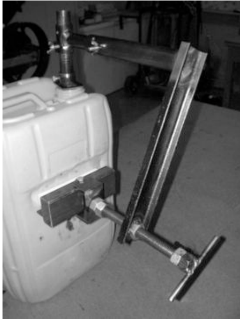
Figure 5.18 Once the heated metal plate has been inserted briefly between the container and the handle (white piece), the pressure screw is ready for immediate tightening.
