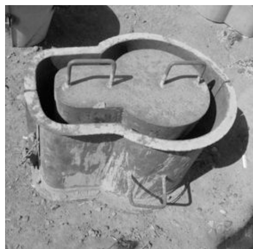
Figure 6.37 The mold built by WaterAid for fabricating the cement latrine seat for the visually impaired.
