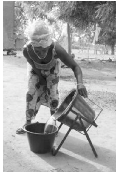
Figure 5.32 Metal bucket tipper being used by a woman having the use of only one arm.
