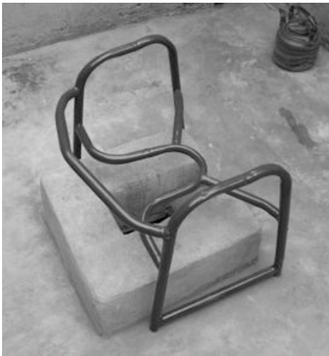
Figure 6.24 Low placed support bracing on the side of this latrine seat makes it more stable and less likely to sink in the ground if used on an earthen surface (such as is found in most traditional latrines).
