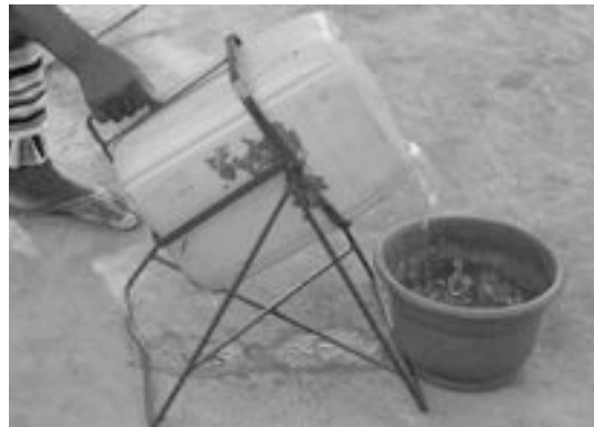
Figure 5.36 Final version of a jerry can tipper being demonstrated.
