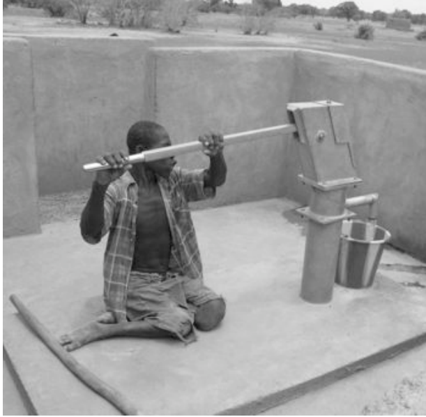
Figure 4.3 This young man finds that he gets more leverage for pumping by sitting on the ground than by staying erect with the aid of his cane. However, since his leverage on the handle is not good, he still struggles to maintain a steady flow rate. At times, the platform floor may be wet or soiled when he comes to use the pump.
