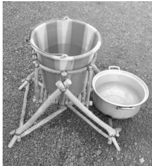
Figure 5.38 One of the final prototypes of the wooden bucket tipper, using local wood attached with thin metal wire.
