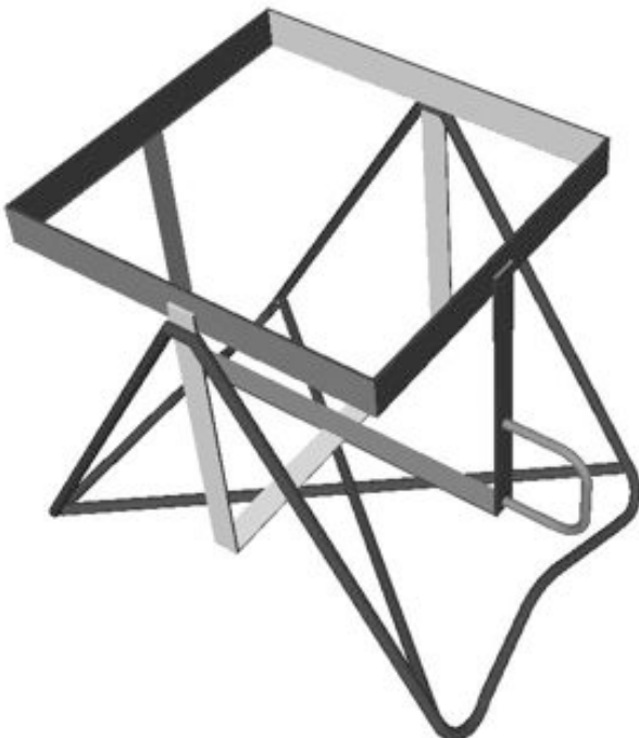
Figure 5.34 Basic design for the metal jerry can tipper, including the rectangular bucket “holder” and the supporting “A” frame base. The holder and A-frame support are joined on either side at a single pivot point.
