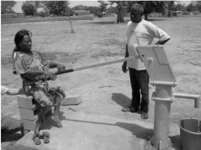
Figure 4.12 A woman with lower-body disability assists with preliminary testing of a T-handle prototype attachment.
