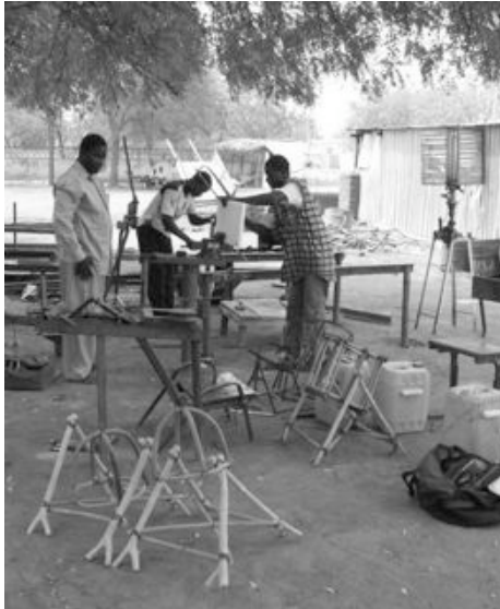
Figure 7.1 A metalworker in Tominan, Mali trains his assistants in aspects of plastic welding, metal container tipper fabrication and the placement of metal pivot sheaths in wooden container tippers. Provision of resources to assist artisans to develop prototypes and to become proficient in fabrication processes of assistive devices can be an important aspect of WASH programs seeking to make such technologies available in local markets.
