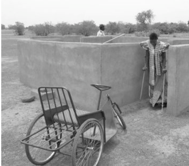
Figure 5.6 Many tricycles for the disabled are built with carrying racks behind the seat; but their height and position behind the seat can make lifting difficult and transport unstable for full water containers.
