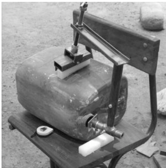
Figure 5.20 The pressure clamp is used by a local metalworker to weld handles to jerry cans for distribution and testing among disabled persons in the target communities.
