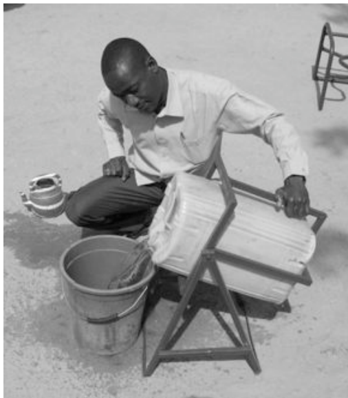
Figure 5.31 Jerry can tipper prototype fabricated in Niger with square, light gauge, iron tubing.
