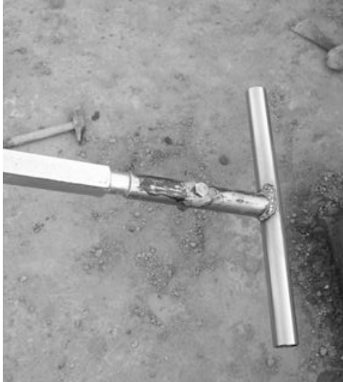
Figure 4.14 The T-handle accessory can be easily fabricated by local metalworkers and is attached to the pump handle with a single bolt. (Note: Use of two, superimposed nuts can serve to reduce the risk of nuts working loose with pump handle use.)
