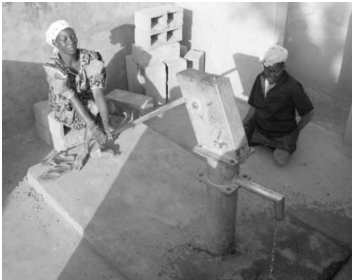
Figure 4.15 Disabled women from the local community assist in preliminary tests of end-seat positioning and height.
