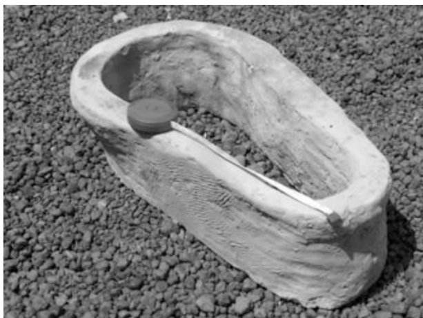
Figure 6.15 Terra cotta (baked earth) latrine seat for sanplat latrines; fabricated by a local potter.
