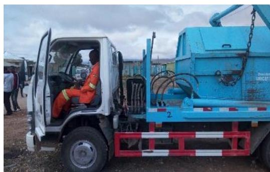
*Photo: A skip loader operating a mechanical arm to lift and transport 5 m<sup>3</sup> garbage bins to landfill sites. (Photo by UNICEF, May 2017)*
