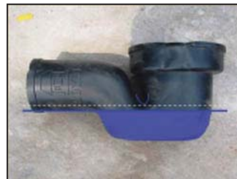
A non-functional siphon like this one fails to make an effective seal and therefore does not protect the users from flies and smells.
