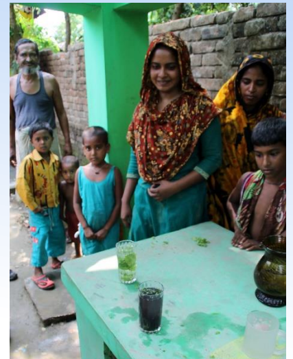
Piped water is tested for arsenic with guava leaves in Mission Para, Satkhira municipality – © Ebo Roek
