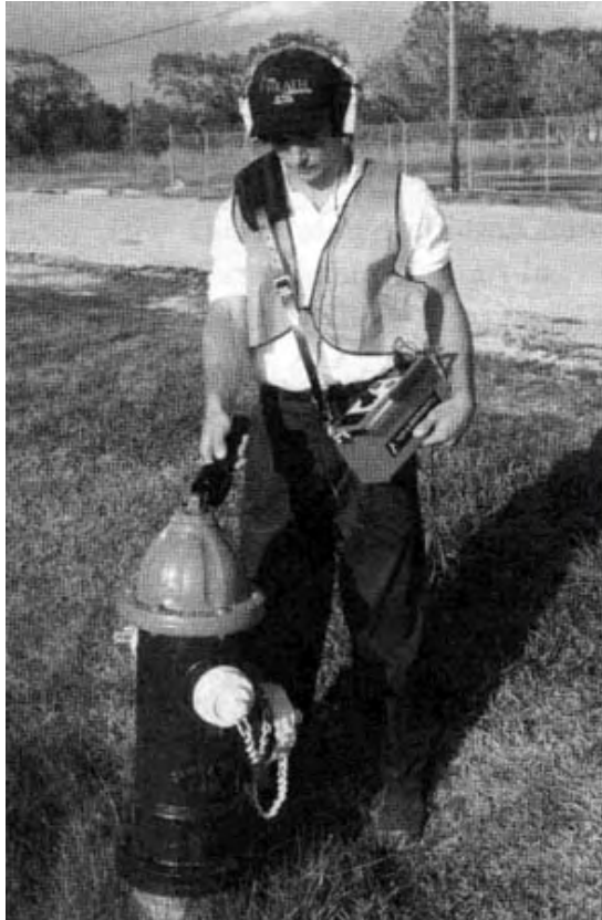
Figure 8-9 Using extension to listen for leak sounds on fire hydrant
