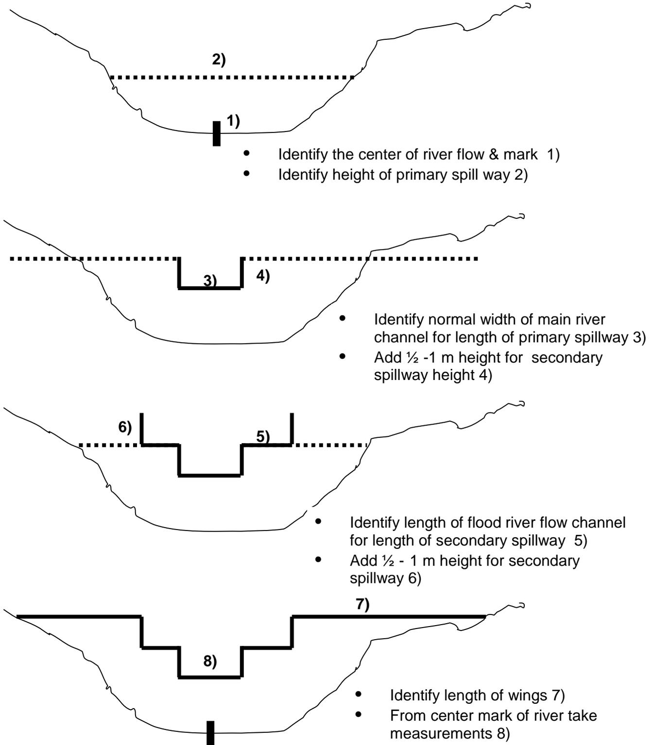
Figure 2. Summary of steps taken to determine sand dam dimensions.
