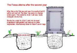
Fig. Fossa Alterna schematic process for second year of use
