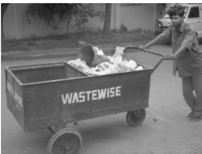
Photo 3. The waste collector is a stakeholder who provides services. His pushcart has two compartments to transport materials separated at source by households (India).
