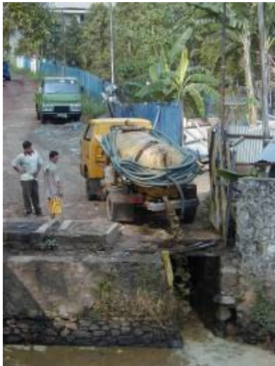
Figure 2: Discharge of septic sludge to river. Source: WSP
