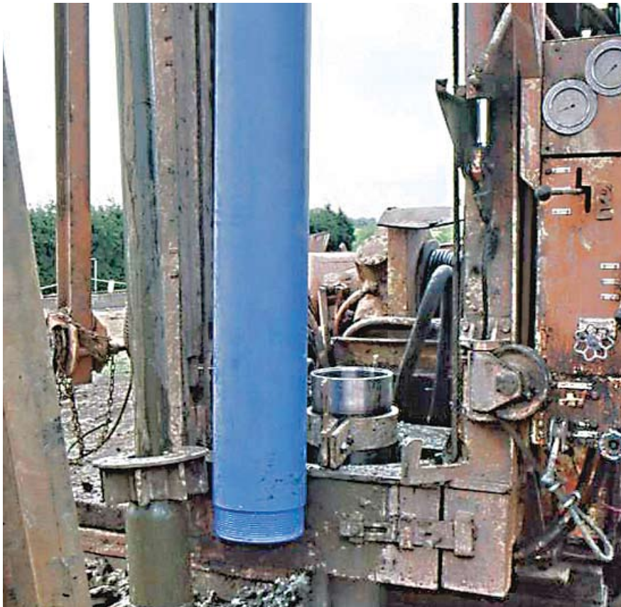
The unit cost of a PVC well casing such as the one shown can be up to 50 percent less than a steel casing
