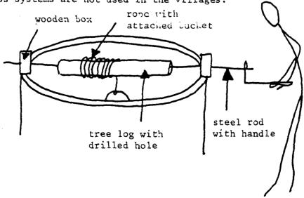
Especially for the wells with water tables below 20 meters the population should be informed about labour saving devices like the rollers or the windlass. For both the building material represent so small costs that there should be no need for external funds. Information and assistance as above.
