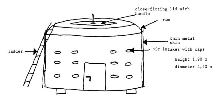
To protect the labourers and keep heat within the kiln a metal skin is clipped to the outside 1 cm from the walls. Also, protective clothing is necessary for the labourer fuelling the kiln from a ladder.
