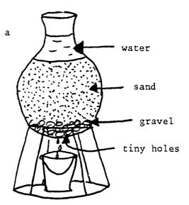
Where measures to prevent water from getting contaminated before it reaches the households fail, purification should take place at a domestic scale. As minimum costs are involved for the use of a jar filter (Sf 1-2 depending upon season for extra jar) the method simple and the material easily available, this measure is regarded as a mere extension matter.
