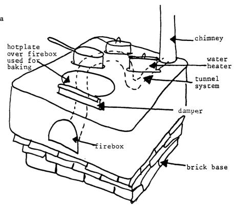
Due to the large masses of clay (non-existant in many parts of the programme area) and water needed, relatively complicated construction and operation and variation from local working practices, the highmass Lorena stove is not recommended for households in the area. It could be tried out at some institutions, however, like El Obeid prison and some of the boarding schools.
