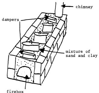
As adobe blocks are quite expensive in the Sudan, and unavailable at village level, experiments should be carried out with the sun-burnt bricks or mud/dung blocks used for construction locally. Also some cement might be needed. Cash outlays for bricks, cement, dampers, chimney and labour would be within the reach of the more well-to-do families only.
