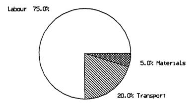
Figure 7. Operation and maintenance cost distribution chart for gravity piped schemes.
