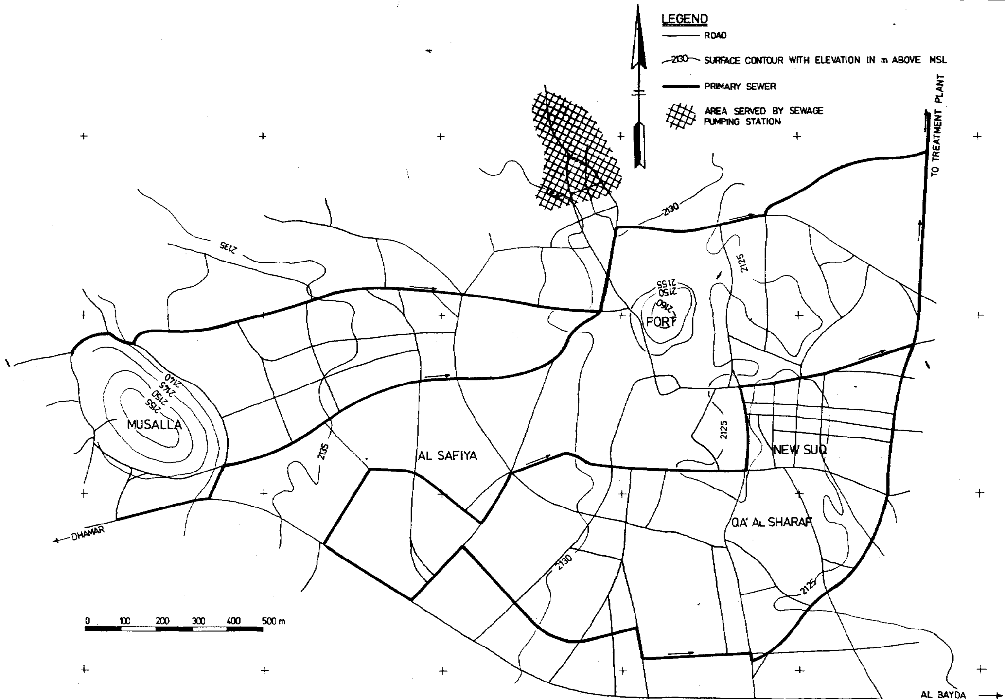
Fig. 3.10. Lay-out of primary sewer system
