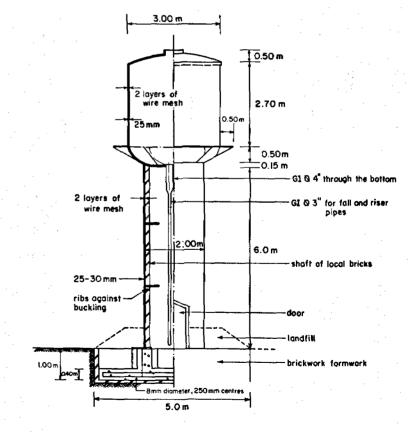
Fig. 2. The ferrocement watertower showing the basic three elements.
