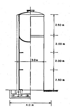
Fig. 10. The improved design. The structure resembles a bamboo.
