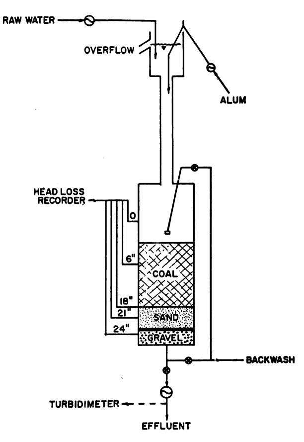
FIGURE 1. Details of Experimental Filter.
