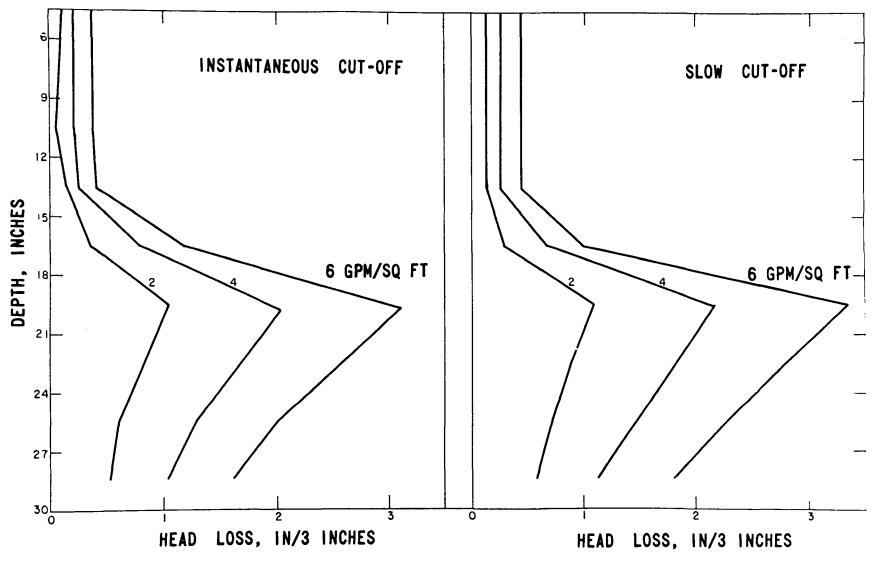
FIGURE 16. Head Loss Gradient, Dual Media.
