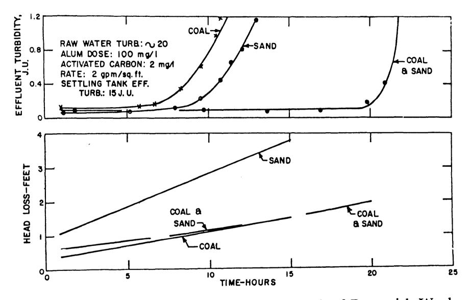
FIGURE 3. Influence of Filter Media on Length of Run with Weak Floc.
