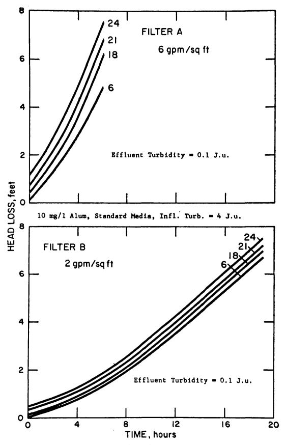
FIGURE 9. Influence of Filtration Rate on Run Length.
