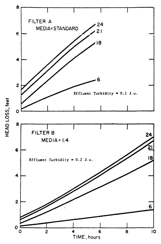
FIGURF 13. Influence of Filter Media on Run Length (4 gpm/sq ft, 10 mg/1 Alum, Influent Turbidity=7 J.u.).
