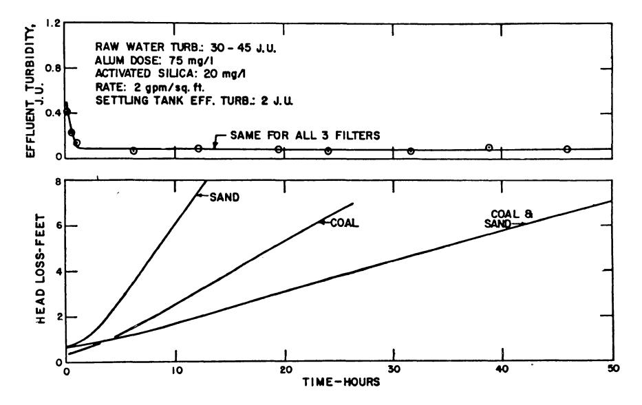
FIGURE 4. Influence of Filter Media on Length of Run with Strong Floc.
