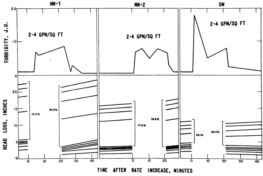
FIGURE 7. Rate Changes with Weak Floc.
