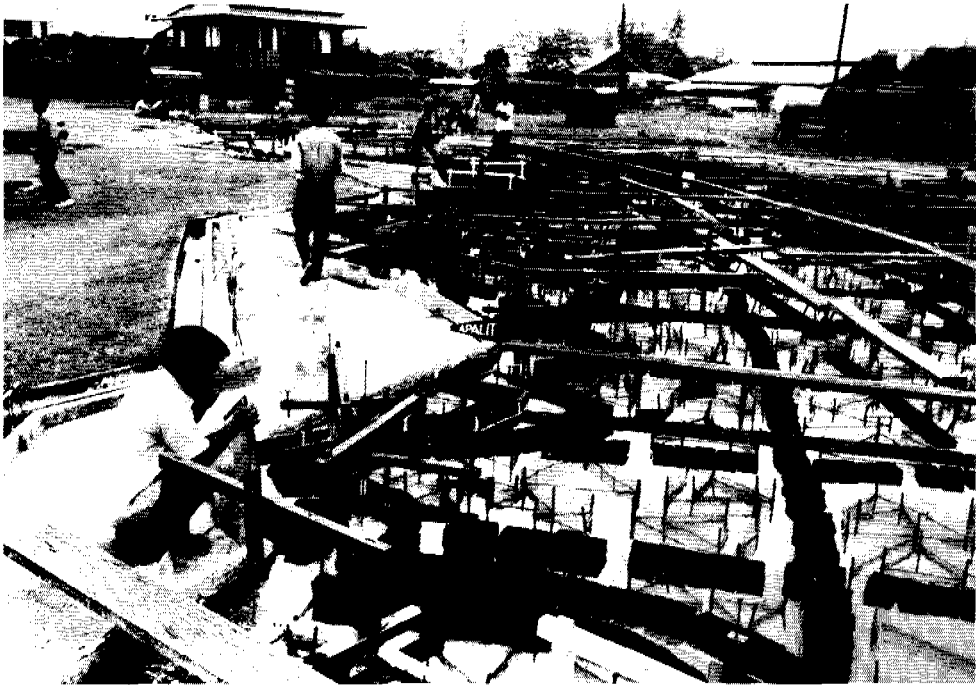
FIG.7 Hydraulic model test in an improvised outdoor laboratory on the flood plain of the Pampanga River, Luzon Island of the Philippines. The objective was to assess the effect of embanking on the maximum flood levels.
