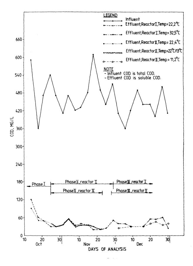
Figure 18. Variation of COD of influent and effluent with time and temperature respectively.
