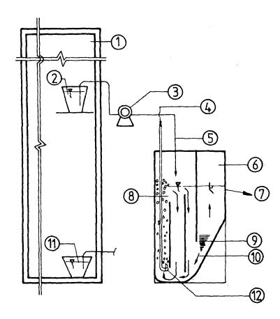
LEGEND 1. Fridge at 4°C (also 10°C for sometime) 2.In fluent container 3. Pump (peristaltic) 4. Air supply 5. In fluent inflow 6. Clarifier (2,11) 7. Effluent outlet 8. Aeration cham ber (7,41) 9. Settled sludge 10.Return sludge flow by gravity 11. Effluent container 12. Aeration nozzle
