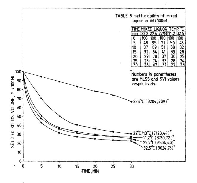
Figure 24. Settleability of mixed liquor solids with time at different temperatures.
