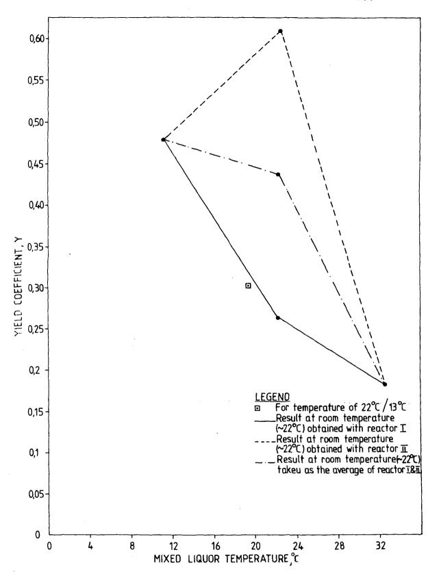
Figure 32. Cell yield coefficient at different temperatures.
