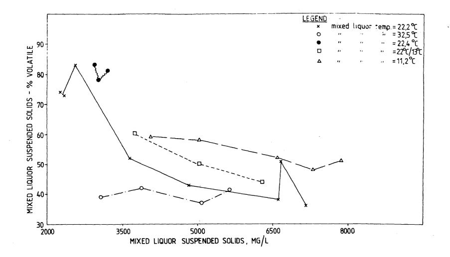
Figure 35. Relationship between the percentage volatile solids in mixed liquor and mixed liquor suspended solids concentration at different mixed liquor temperatures.
