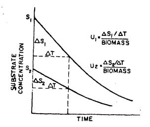
Figure 12. Determination of specific utilization rate from a batch culture /29/. If equation 4.8 is inverted and rearranged it would assume an expression:
