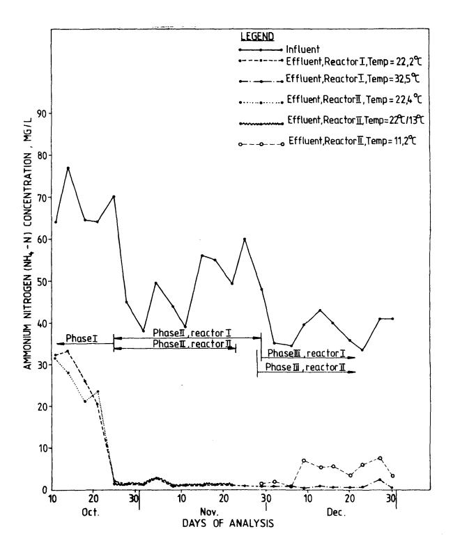
Figure 20. Variation of ammonium nitrogen  $(NH_4-N)$  concentration in influent and effluent with time and temperature respectively.
