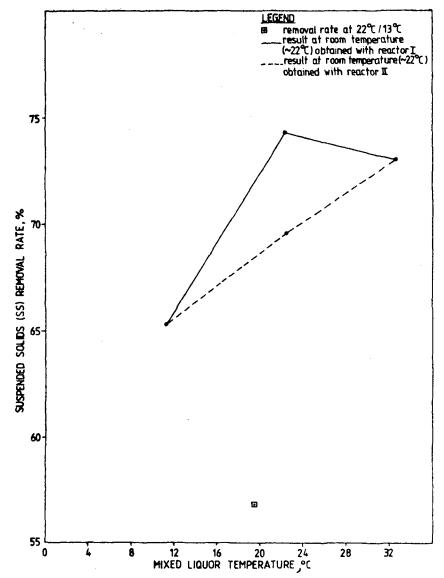
Figure 23. Suspended solids (SS) removal mates at different temperatures.
