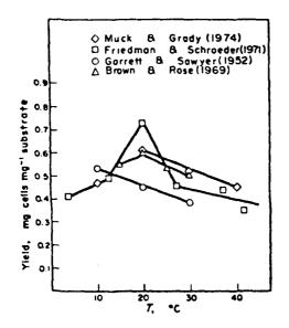
Figure 31. Variation of the true cell yield coefficient with temperature /6/.
