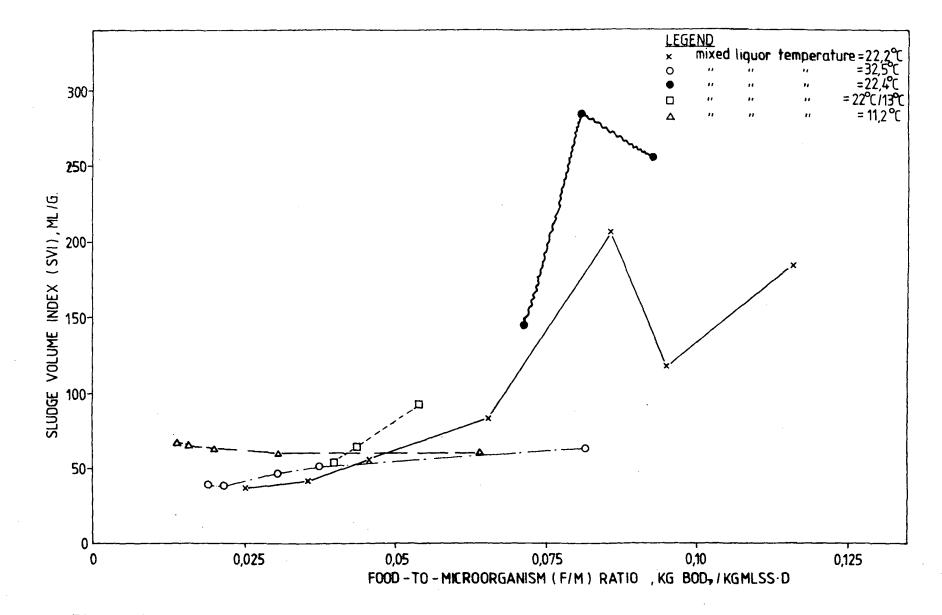
Figure 25. Relationship between sludge volume index (SVI) and food-to-micro-organism (F/M) ratio at different mixed liquor temperatures.
