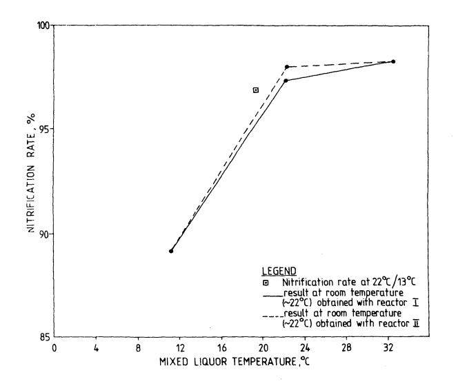
Figure 21. Nitrification rate at different temperatures.
