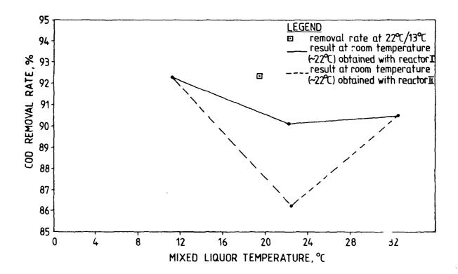
Figure 19. COD removal rates at different temperatures.
