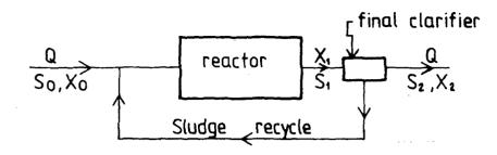
Figure 10. Flowchart of continuous flow system of CMAS process.
