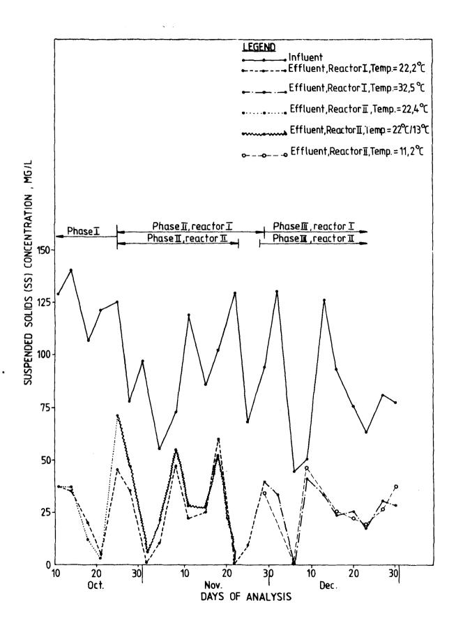
Figure 22. Variation of suspended solids concentration in influent and effluent with time and temperature respectively.
