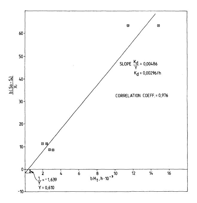
Figure 28. Determination of yield coefficient (Y) and specific organism decay rate  $(K_d)$  for temperature of 22,4°C.
