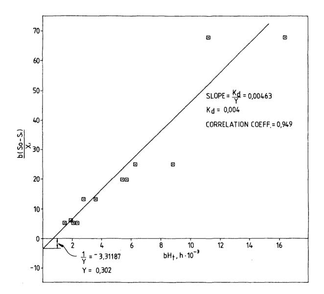
Figure 29. Determination of yield coefficient (Y) and specific organism decay rate (K<sub>d</sub>) for temperature of 22°C/13°C.
