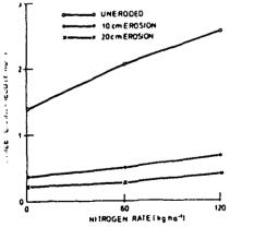
Maize grain yield from a desurfaced Alfisol at .hree levels of N fertilizer application.
