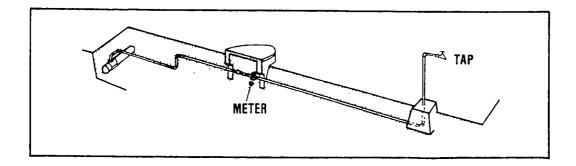
Public standpipes have long been in use in supplying water to communities owing to their cheap cost and technical feasibility. They are usually made of masonry, brickwork or concrete. A service pipe is built through the structure and is connected to one or more taps. Figure 2 shows a typical cross section of a multiple-tap standpipe.
