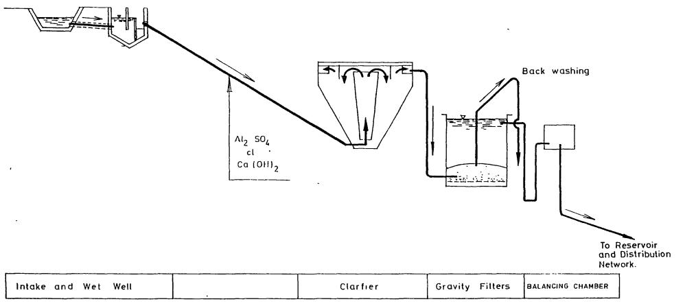
Figure 7. Schematic view of the treatment plant in Awassa (GWE, 1978).
