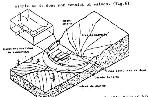
The surface area of the catchment in the "CAPTSA EARTHEN DAM" is in the order of 3 hectares, the slope should be equal to or larger than 2%. Preferably, the catchment area should be chosen in soils which are shallow, rocky and thus unsuitable for agriculture. This reduces the risk of erosion and also allows a better runoff which can be increased by artificial handdug drains where necessary.
