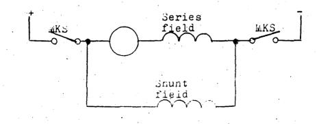
The simple circuit representing the end result of a controller
