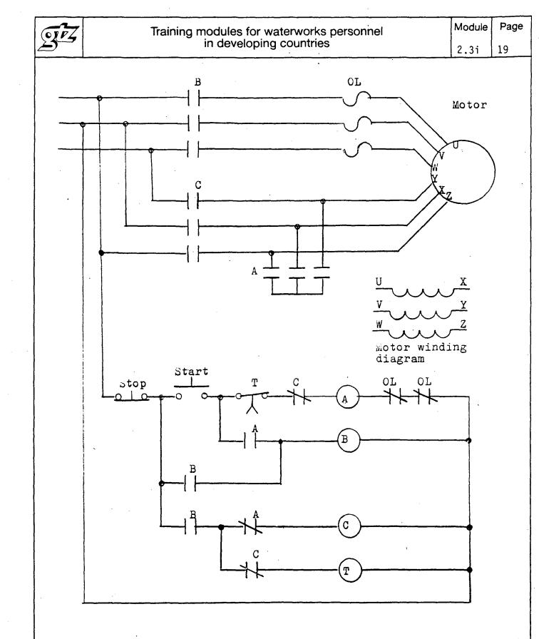
Fig. 17 - Typical star-delta starter schematic for a three phase squirrel cage motor.
