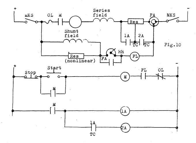
If the motor speed range is more than 2 to 1, the presence of a field rheostat creates two demands on the controller.
