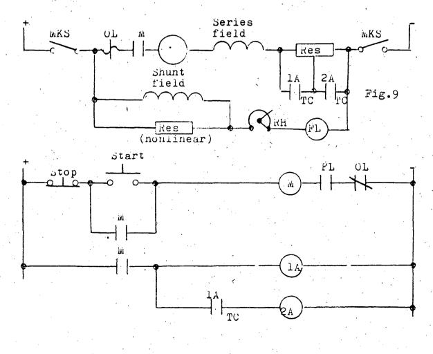
When a motor is shunt wound or lightly compound wound, its speed can be increased above rated base speed by decreasing the strength
