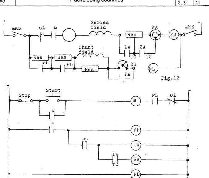
started and running, the relay coil is energized, thereby shorting out the economizing resistor.
