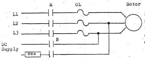
Fig. 11 Simple power circuit for dynamic braking of a squirrel cage motor.
