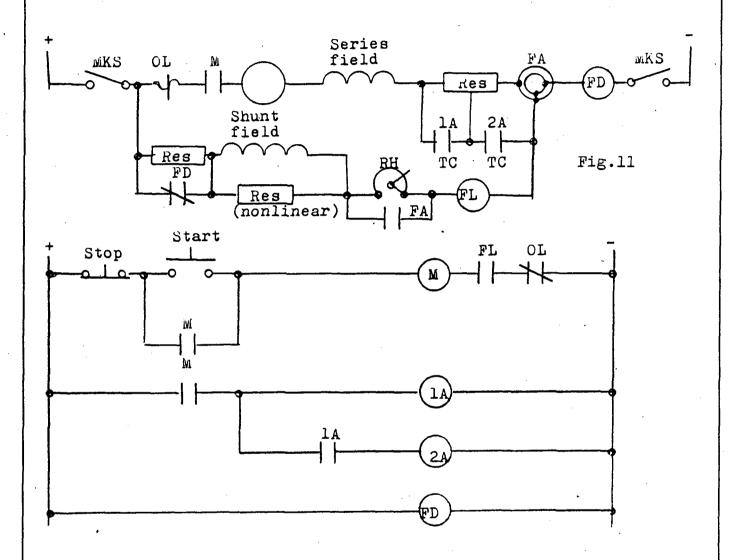
Reversal current can be held to an acceptable value with a field decelerating relay, FD and an associated resistor. The type of relay shown in the circuit has a series coil, which is connected in the armature circuit, and a shunt coil, which is connected across the control-circuit supply. The relay also has a normally closed contact which is connected across the resistor in the shunt field circuit.
