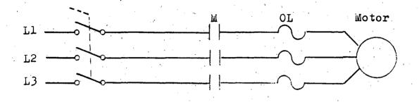
Circuit for combination starter with disconnect switch.
