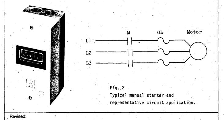
The thermal protective device which is normally an integral part of all motor starters is designated by the symbol "OL" (overloadrelay) on the circuit diagrams. It consists of two to three heaters in series with the motor circuit to be protected, above these heaters are strips of bimetallic material, which act as latches for the contact members. Bending of the bimetallic strips under heating of overload current will release the latches and allow the contacts to open.
