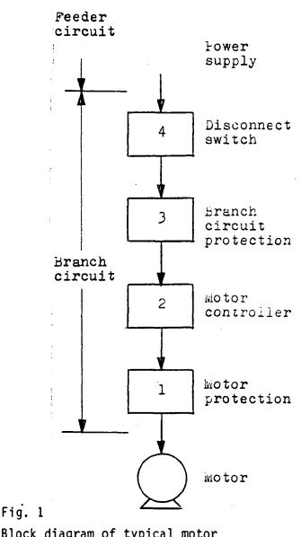
Block diagram of typical motor branch circuit.
