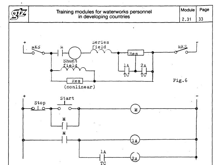
This condition would be unacceptable in most cases. The solution would be to reduce, or cut out, resistance after the motor had reached an appreciable speed. Thus, the motor would eventually be able to attain normal speed when no external resistance remained in the circuit. This result is accomplished with accelerating contactors.
