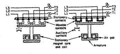
(a)-Coil de-energized, main contacts open. (b)--Coil-energized, main contacts closed.
