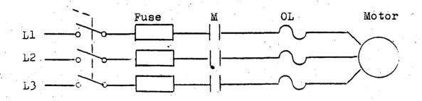
Circuit for combination starter with fused disconnect swith
