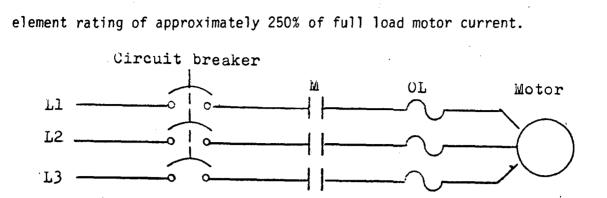
Circuit for combination starter with circuit breaker
