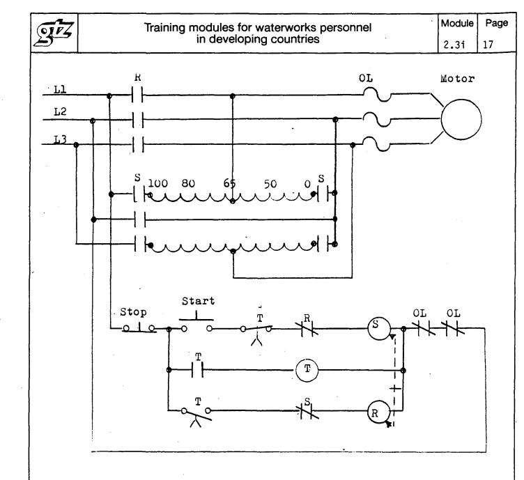
Fig. 16 - Typical autotransformer starter schematic for a three phase squirrel cage motor.
