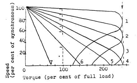
Fig. 21 Speed-torque curves for values of resistance indicated on curve of starting torque in Fig. 20
