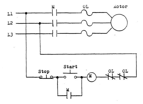
Fig. 6 Circuit diagram of across-the-line starter and momentary-contact pushbutton for providing low voltage protection.
