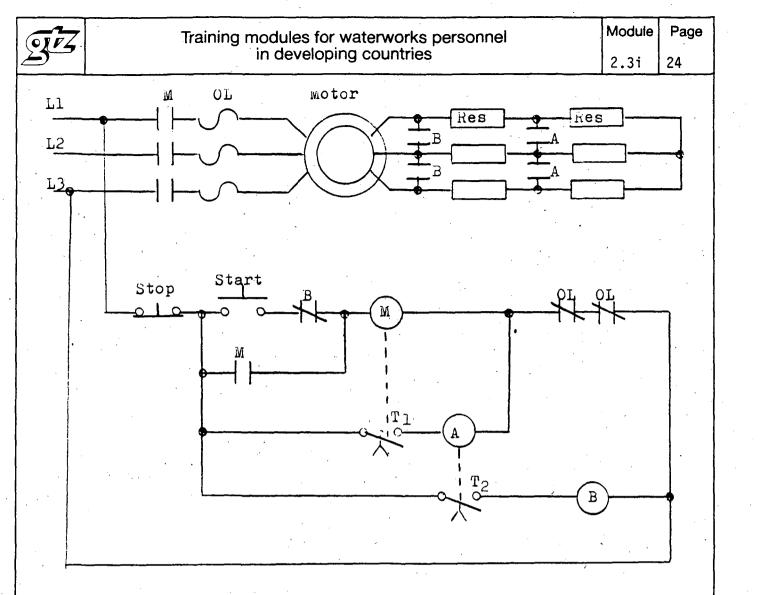
Fig. 22 - Typical magnetic starter schematic with 3 step acceleration for wound-rotor motors.
