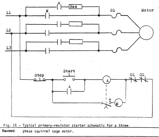
When the start button is pressed, contactor A closes and applies power to the motor through the resistors. Timer A begins to time out and closes after the proper time interval. When the timer contacts close, M contactor is energized. The M contacts short out the resistors and apply full voltage to the motor.
