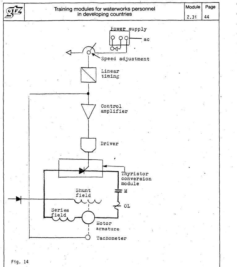
One-line-diagram showing self-contained dc Motor controller with ac-dc conversion and variable dc voltage control.
