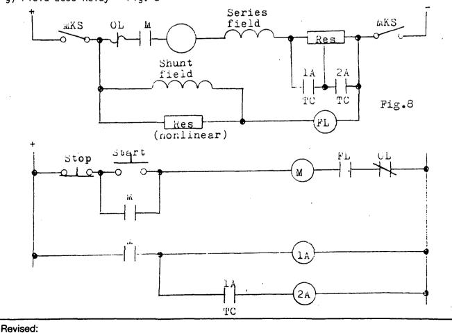
Another fault condition that must be sensed and acted upon is the loss of shunt-field excitation. Otherwise, the motor will tend to run away. At the same time, the motor will draw a high current from the power supply. Either mechanical damage or electrical damage, or both, could result from this condition.
