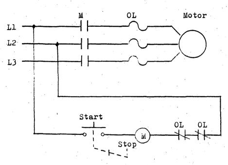
Fig. 5 Circuit diagram of across-the-line magn. starter and maintained contact push-button for providing low voltage release.
