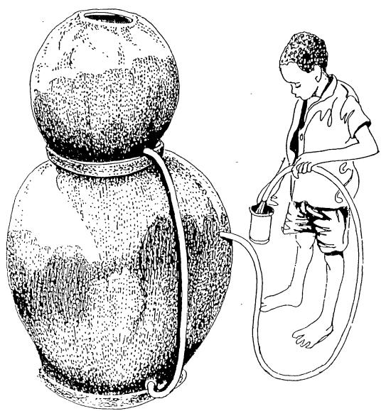
The Upward Flow Water Filter is an easily built family size water filter suitable for removing suspended particles of soil or organic matter which discolour or pollute drinking water. The filter is particularly useful in rural areas where surface water of doubtful quality is often used. The use of clean water can contribute significantly to improving family health.
