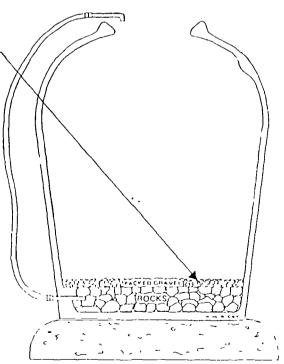
on a low table) and connecting it by hose with the inlet of the filter. Water is allowed to flow from the storage tank to the filter tank until it reaches the top of the filter bed being checked. It is important that this procedure is repeated after
