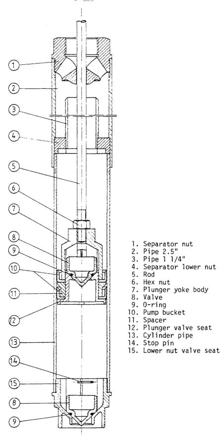
Figure 2.3 Particle separator designed to fit the SWS cylinder.
