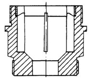
Figure 3.3 The plastic foot valve designed for machining.
