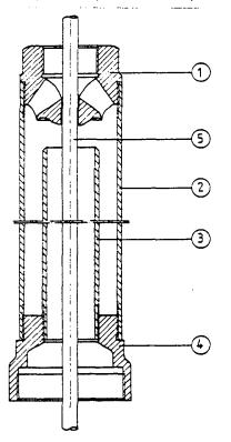
Figure 2.2 Particle separator designed to fit the India Mark II cylinder.
