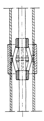
Figure 4.1 Design of the pump rod guide.
