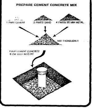
1 PART CEMENT, 2 PARTS SAND, 4 PARTS 20 MM METAL MIX THOROUGHLY & POUR CEMENT CONCRETE UPTO 8 CM INTO THE PIT.
