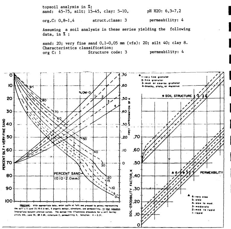
The soil-erodibility nomograph. Where the silt fraction does not exceed 70 percent, the equation is 100 K = 2.1 M<sup>1.14</sup> (10<sup>-1</sup>) (12 - a) + 3.25 (b - 2) + 2.5 (c - 3) where M = (percent si + vfs) (100 - percent c), a = percent organic matter, b = structure code, and c = profile permeability class.
