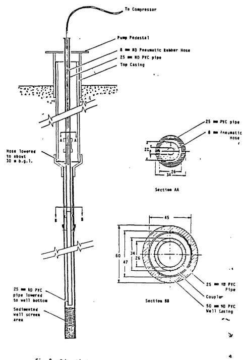
Fig. 9 : Schematic Layout of Well Cleaning Procedure using 25 mm ND PVC pipe and 8 mm ND pneumatic hose
