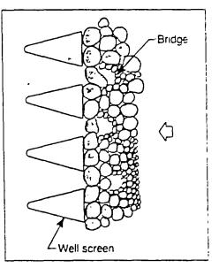
Figure 15.4. During development by overpumping, sand grains can bridge openings because fices occurs in only one direction. Once the well is placed into service, agitation by normal pump cycling can break — whithe bridges, causing sand pumping.
