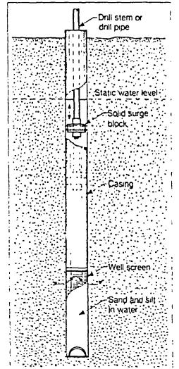
Figure 15.7. For certain types of formations, a surge block is an effective tool for well development. On the downstroke, water is forced outward into the formation: water, silt, and fine sand are then pulled into the well screen during the upstroke.
