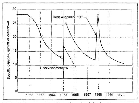
Figure 19.9. Performance record of a well in New Jersey shows declines in specific capacity caused by the growth of iron bacteria, and recovery of specific capacity produced by periodic treatment. Shock treatment with chlorine once a year would help maintain the yield at a satisfactory level. A. C. Schutters Company)
