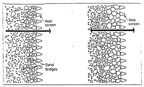
Figure 15.5. Effective development action requires movement of water in both directions through screen openings. Reversing flow helps break down bridging of particles. Movement in only one direction, as when pamping from the well, does not produce the proper development effect.
