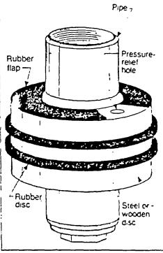
Figure 15.6. Typical surge block consisting of two leather or rubber discs sandwiched between three steel or wooden discs. The blocks are constructed so that the outside diameter of the rubber lips is equal to the inside diameter of the screen. The solid part of the block is 1 in (25.4 mm) smaller in diameter than the screen.
