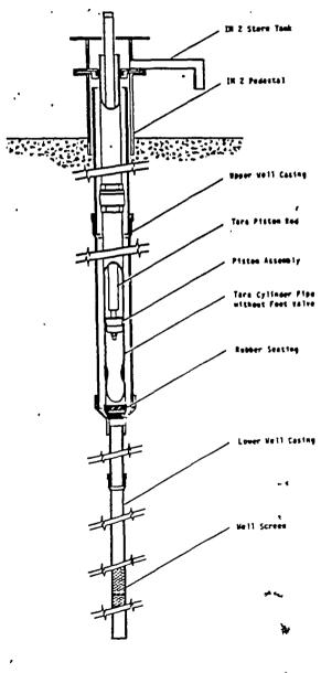
Fig. 8 : Manual Well Cleaning & Over pumping using the Tara DA Pump components
