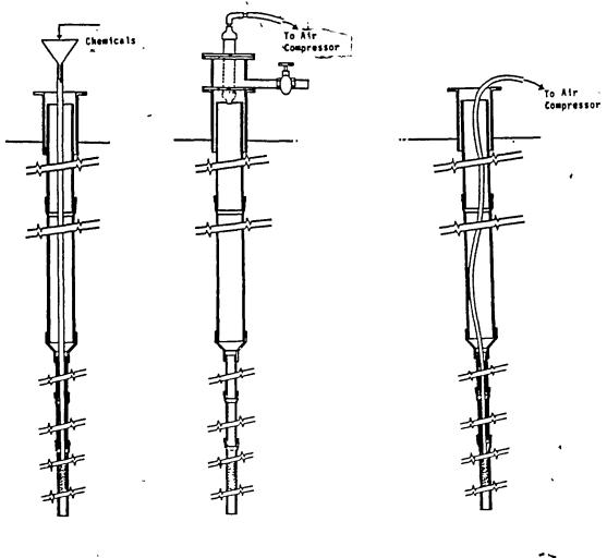
Fig. 7.1 Placement of Chemicals Fig. 7.2 Pressurising the Well Fig. 7.3 Well Cleaning & >> Over pumping by Air-lift
