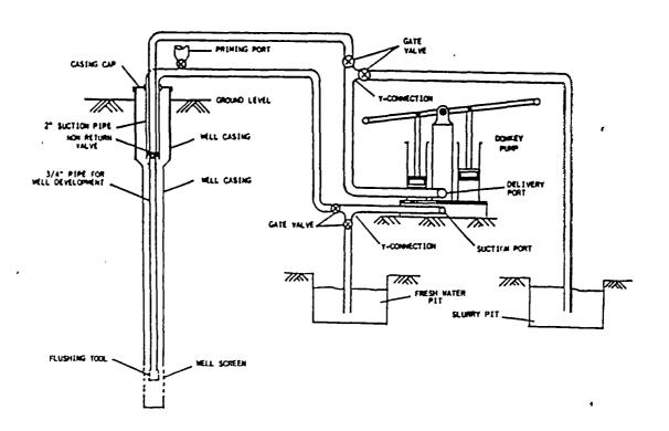
Fig. 6 : Schematic Layout for Water Injection & Over pumping with Donkey Pump
