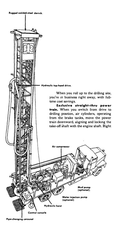
away all drilling systems are "go". Engine power is now being transmitted directly to the air compressor, gear case and hydraulic pumps. You get full horsepower for all drilling functions and save fuel whenever the rig is running.
