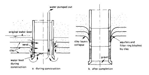
Fig. 21. Blocking of aquifer and filter rings by collapsed clay layers.
