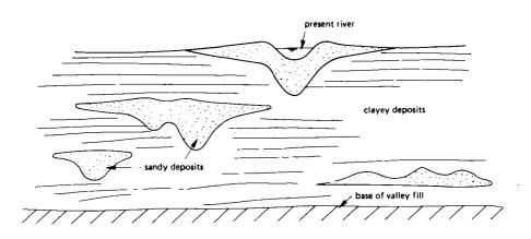
Fig. 5. Schematic geological cross-section over river valley
