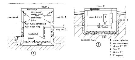
Fig. 16. River well with rings in river and pipe to the bank
