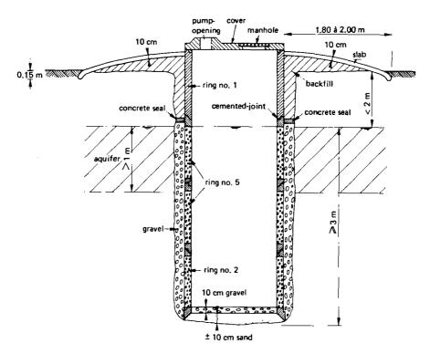
Fig. 17. Standard well (type A)
