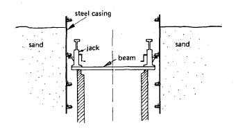
Fig. 20. Removing steel casing with jacks.
