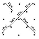
Fig. 10. Drilling pattern in wet places
