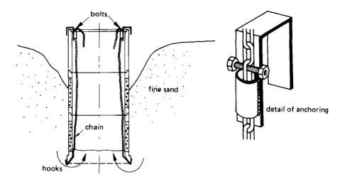
Fig. 19. Preventing uneven setting of well rings
