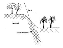
Fig. 6. Schematic geological section over fault zone
