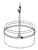
Fig. 30. Sling for turning over a concrete ring
