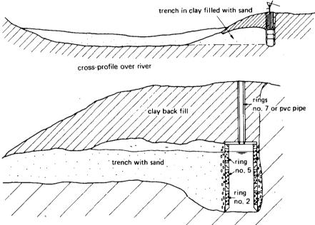
Fig. 15. River well with sand trench to the bank
