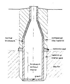
Fig. 25. Well with in-situ brick lining.
