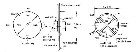
Fig. 23. Details of simple mould for concrete rings.
