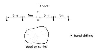
Fig. 7. Survey pattern near pool or spring
