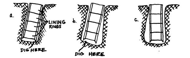
Figure 8-9. Straightening well rings in loose soils./5/
