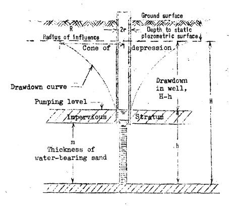
Figure 1-2. Diagram of well in artesian aquifer showing the meaning of various terms used in the equilibrium formula.
