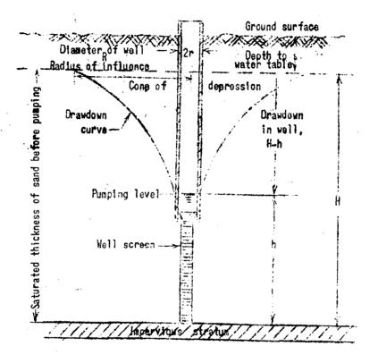
Figure 1-1. Diagram of water-table well showing the significance of the various terms used in the equilibrium formula.
