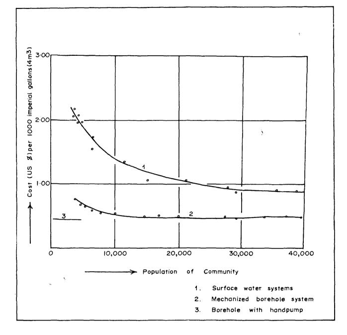
Figure 5. Comparative cost of developing surface water mechanised borehole and borehole with handpump [6].
