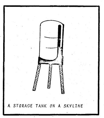
from storage tanks where it had been stored during an earlier low-use period. For example, at night the demand for water is lower than during the day. The system is still capable of delivering large quantities of water, however, because this water is in excess of the night time needs, it can be stored in tanks to be distributed the following day during the peak-load periods.
