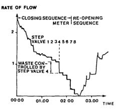
Fig. 5. Flow rate during step test
