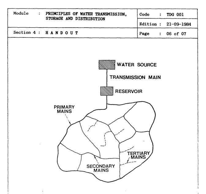
Fig. 7. Schematical lay-out of distribution system.
