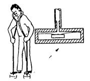
Fig. 2. Sounding for water leaks: - with electronic sounding equipment (left and middle); - with acoustic geophone (right).
