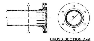
Fig. 1. Thrust at end of pipe.
