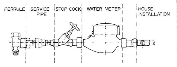
Fig. 1. Typical service connection assembly.
