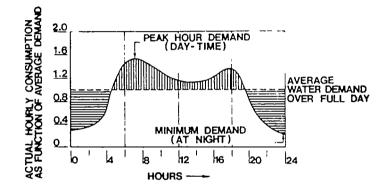
Fig. 4. Daily fluctuation of water consumption.
