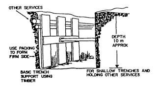
Fig. 2. Supporting trench sides
