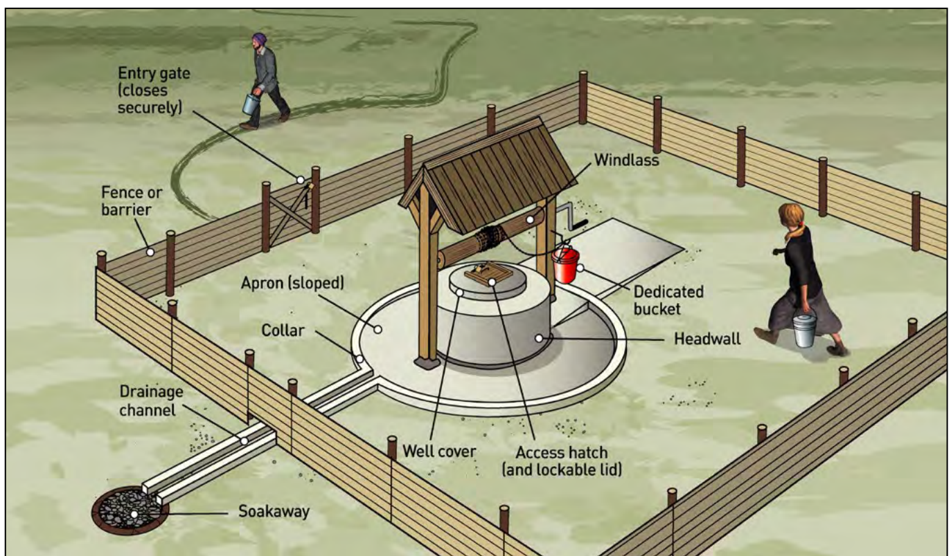
Figure 1. A common dug well with a windlass in a sanitary condition
