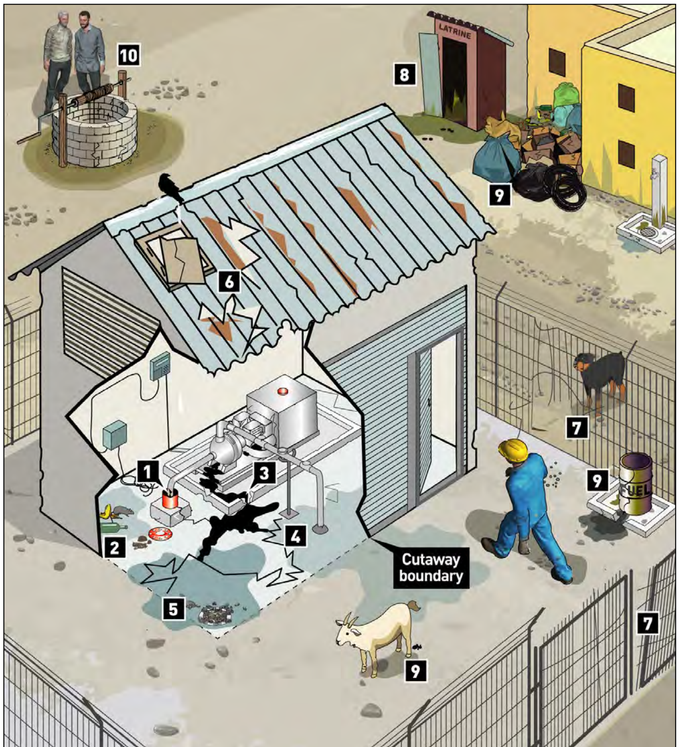
Figure 1. Typical risk factors associated with a borehole with a motorized pump
